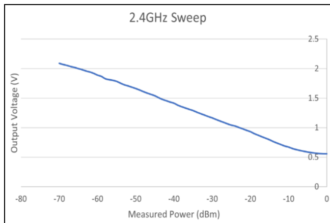
Fig 1: 2.4GHz power sweep for the AD8318 logarithmic amplifier
