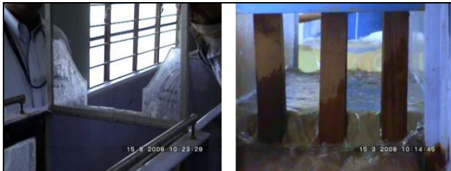
Experimental condition under Artificial Tail Water Submergence of 60 – 70% in the Laboratory Flume
