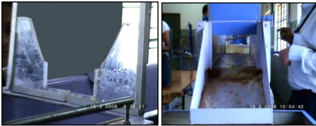
Experimental condition under Natural Tail Water Submergence of 40 – 50% in the Laboratory Flume
