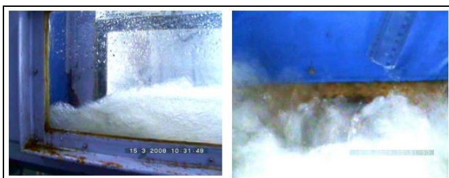
Photographs showing hydraulic jump formed very close to the sluice gate (Section and Plan)
